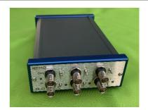
The 3X-CI is a 3 channel IEPE and charge signal conditioning unit, housed in a compact and rugged chassis. Featuring DC power input it can be used via the supplied mains DC adaptor or via a field based DC supply such as battery.
