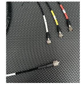
The 7F81-30 is a 3m cable assembly developed for use with a range of triaxial accelerometers that use a 1/4-28UNF threaded 4 pin connector. This connector is used on several of Kemo's own accelerometers as well as on a wide range of other competitor products.
